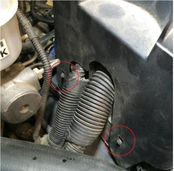
Remove the 4 bolts holding the fender brace and unclip the fusebox cover from the 2 retainers towards the bottom (circled).
