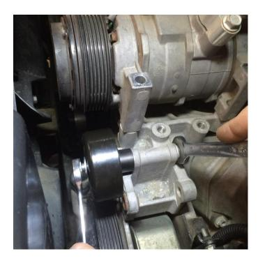
Install the idler pulley and spacer into the open boss of the factory bracket.
