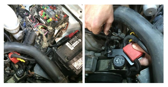
Route the positive battery cable lead underneath the upper radiator hose as shown and then reconnect to the battery and fusebox. The fusebox cover, lid, and fender brace can be reinstalled. The junction box will snap into the new supplied bracket and bolt on with the original bolt.
