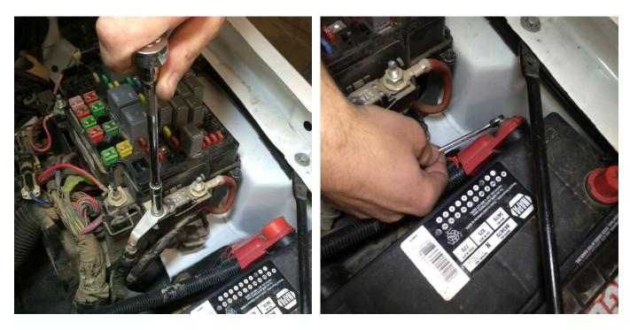
Disconnect the negative battery terminals on BOTH batteries (not shown), then remove the fusebox power wire and the positive terminal on the battery as shown.
