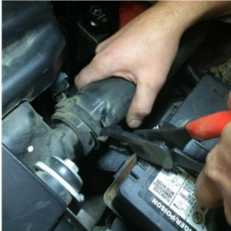
Remove tension from the upper radiator hose clamps. They can be locked into themselves in the open position. Break the seals and slide the hose out approximately  $\frac{1}{4}$ " on each water neck
