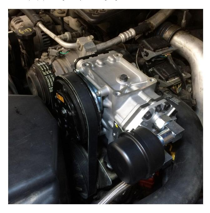
There are multiple positions in which the compressor can be mounted based on your application. If space allows, vertical mounting is always preferred for the least amount of oil bypass. **SLM compressors can only be mounted vertically**. Please refer to the chart below to determine which position is to be used. These instructions describe the horizontal mounting. Please refer to the 2007-present instructions for vertical mounting.
