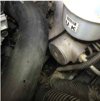
Check clearance at the head fittings and behind the hose to the master cylinder. The hose needs to be manipulated until it has the most average space to any object. Now is a good time to start the engine and verify there are no problems with the serpentine drive, and that the compressor is not visually out of line.
