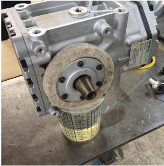
**Standard Compressors:** Verify the new compressor has the half-moon shaped woodruff key installed in the crankshaft. The compressors are shipped pre-filled with AC refrigerant oil, but it is recommended to run 12oz of SAE 30 non-detergent engine oil. Remove the bolts from each side of the compressor fill ports and drain the oil.
