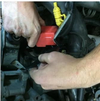
Installation of this system requires shifting the battery junction box into a new position with the supplied hardware. Remove the bolt holding the factory bracket and unclip the junction box from the bracket.
